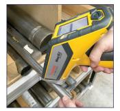
All raw materials and castings are PMI tested on receipt to validate material specification and ensure the highest quality in each component.
